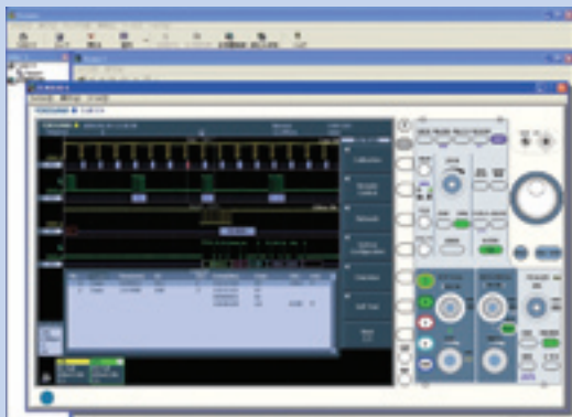
Control a DLM6000/DL6000 via USB or Ethernet. Provides simple control and transfer of waveform data to a PC through an intuitive man-machine interface.
