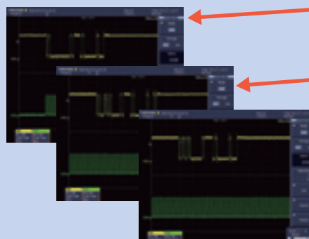
By using History memory, up to 2000 waveforms of just the command portion (CMD) are held.
