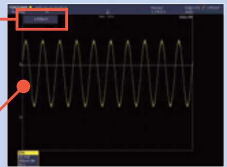
Trigger levels are magnified during adjustment for ease of reading
