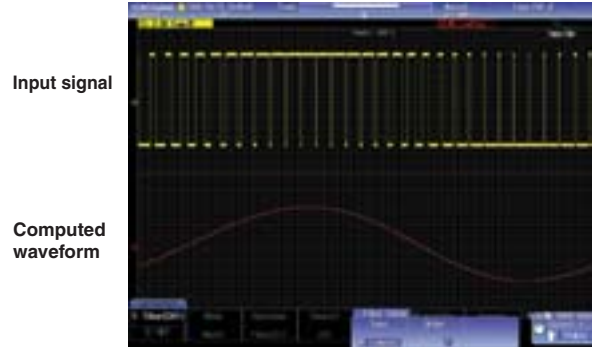
Filtering of a PWM waveform using computation
